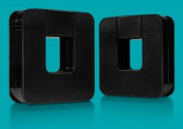
Ideal for gathering high-precision measurements in commercial or industrial electrical panels or switchgear, the AcuCT mV Series is a revenue grade current transformer with a safe, 333mV output. The AcuCT mV is compatible with a range of meters or other instrumentation and the pull-apart, split-core design helps facilitate fast installation without cable or wire disconnection.
