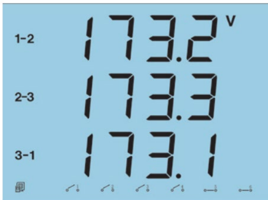
Fig 3.3 Line to line voltage
