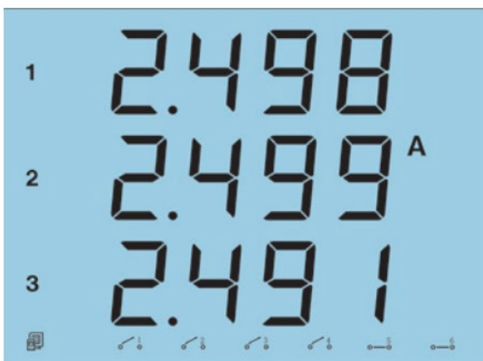
Fig 3.4 Three phase current
