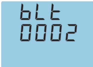
Fig 3.27 LCD back light time setting
