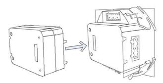
The AXM-WEB-PUSH module is linked to the Acuvim II series meter by a communication plug. Other extended modules such as the IO modules can be linked to the Acuvim II series meter through the AXM-WEB-PUSH.
