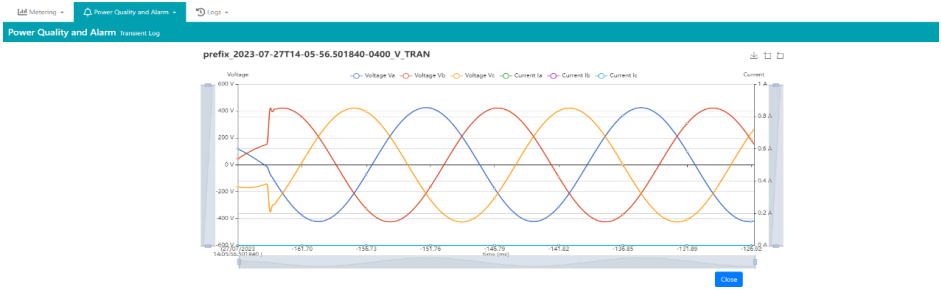
Figure 6-15 Transient Voltage View Webpage
