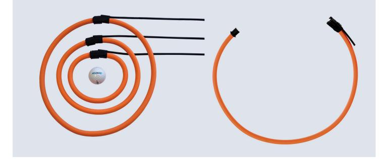
Accuenergy's flexible Rogowski coil is designed for use where regular solid or split core current transformers cannot fit, and is ideal for power quality monitoring such as harmonics. Advantages of the Rogowski coil include; high accuracy, wide measurement and frequency range with no additional integrator or power supply needed.
