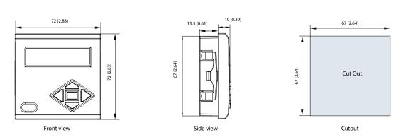
Display Module is designed with flexibility in mind, it can be installed together with the base unit or can be mounted on a panel.\* \* (when ordered as a separate module. Please see ordering information for details).
