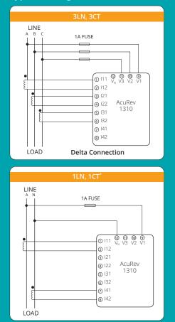
LINE 1A FUSE 10 10 0 0 V<sub>N</sub> V3 V2 V1 111 @ 112 -3 121 AcuRev 4 |22 1310 © 131 6 132 @ 141 8 |42 Direct Connection, without PT's LOAD
