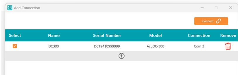
**Figure 4-6 Connecting AcuDC 300 to Acuvue 2 through Modbus RTU**
