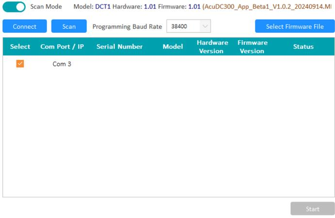
**Figure 4-27 Update the Firmware via Modbus RTU**
