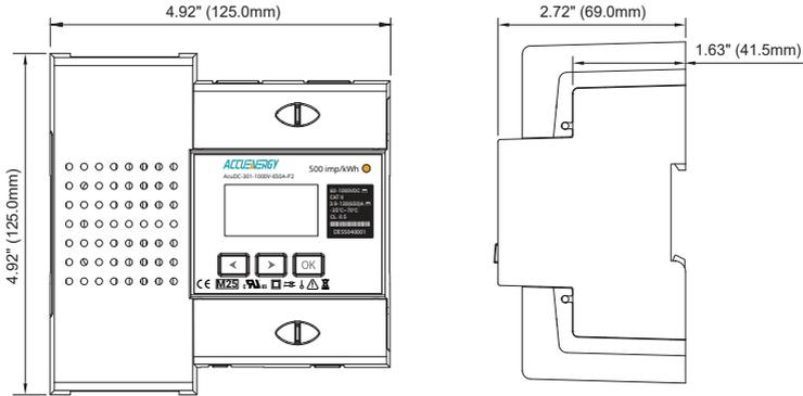
**Figure 2-1 AcuDC 300 Front and Side View Diagram**
