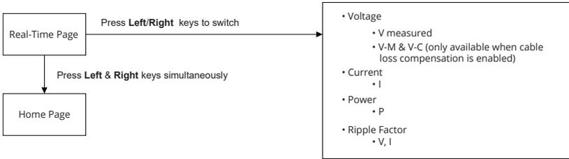
Figure 3-4 Real-time Display Screen Structure
