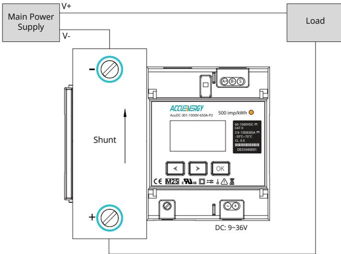
Figure 2-7 AcuDC 300 Current Wiring
