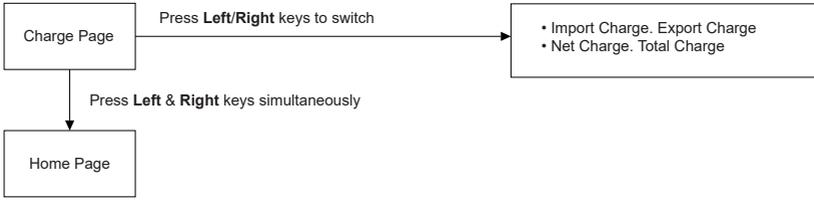
**Figure 3-15 Electrical Charge Screen Sequence**
