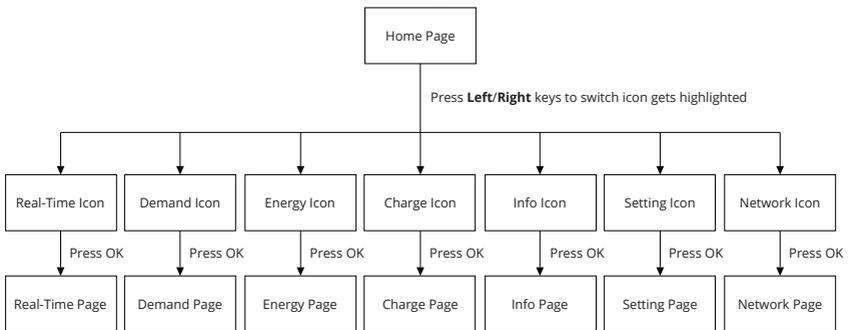
Figure 3-2 Navigation Structure of AcuDC 300 Display Screen
