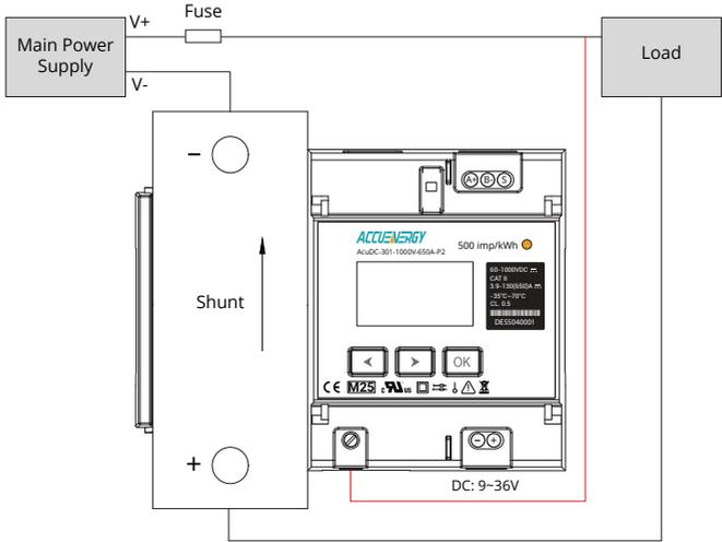
Figure 2-6 AcuDC 300 Voltage Wiring
