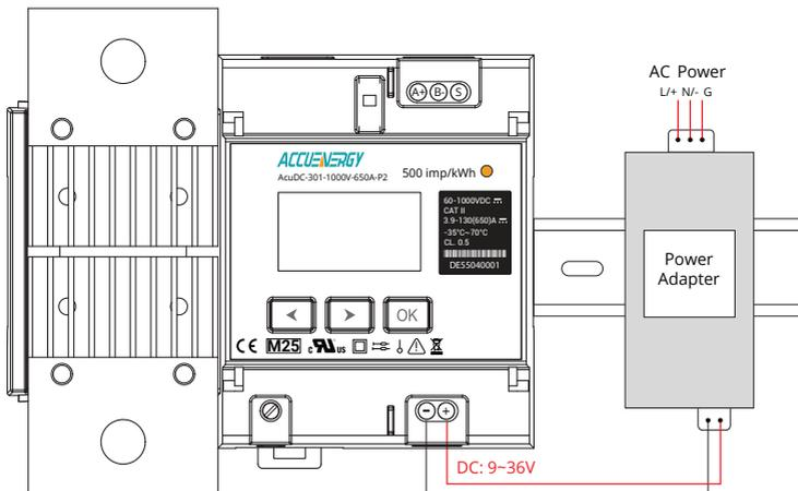
Figure 2-5 AcuDC 300 Power Supply Wiring
