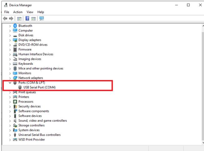
Figure 4-4 COM Port Number Assigned to RS485-to-USB Converter
