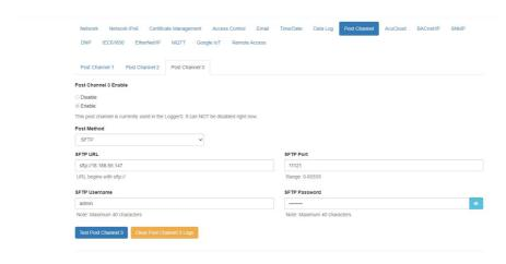
Click the 'Save' button after changing any settings. Users will be prompted to reboot the AXM-WEB2 series module immediately or at a later time. If later is chosen the AXM-WEB2 series module must be rebooted from the 'Management' page for the settings to take effect.
