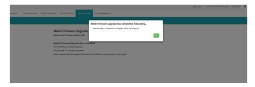
After the meter reboots, users will be able to log back into the web interface. When logged in, click on the 'About' navigation tab located on the top right corner of the web page to view the 'Device Information' page. Users can check this page to confirm the meter's firmware version was updated correctly.
