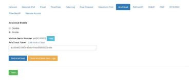
**NOTE:** The "TEST AcuCloud" button should only be utilized after clicking the 'Save' button otherwise a failure response will be observed. If a failed response occurs after clicking 'Save', please double check the serial number entered in AcuCloud, the token entered in the web page as well as viewing the test post details by clicking on the 'Details' option.
