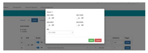
Once all alarm settings are configured, user must click on the 'Save' button and then reboot the communications module for the settings to take effect.
