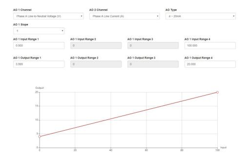
The interface displays a graph for the analog output signal according to the input range that has been configured.
