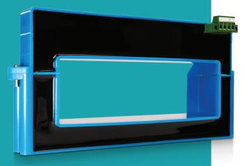
The HAB Series Hall effect DC current sensor is designed to measure up to 5000A of DC current with 0.5% accuracy. Designed to adapt, the HAB is available with either 4-20mA or 0-5V output and as either a uni-directional or bi-directional device for broad compatibility. Suited for existing applications, the split-core design can be installed without wire or cable disconnection
