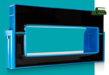
The HAB Series Hall effect DC current sensor is designed to measure up to 5000A of DC current with 0.5% accuracy. Designed to adapt, the HAB is available with either 4-20mA or 0-5V output and as either a uni-directional or bi-directional device for broad compatibility. Suited for existing applications, the split-core design can be installed without wire or cable disconnection
